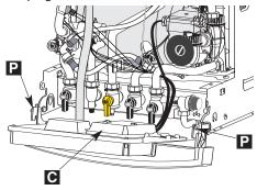
the earth plug from the earth socket. Hang out the main PCB. Reassemble in reverse order.
