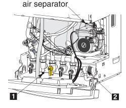
1 = DHW circuit drain point
