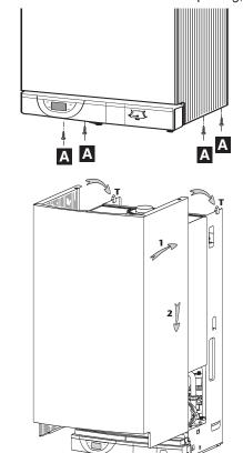
carefully locate on lugs  ${\bf T}$  on the top edge of the chassis.
