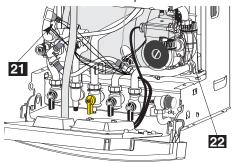
the plug, remove the retaining clip pull the thermistor out. Reassemble in reverse order.
