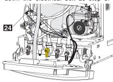
Disconnect the 2 cables, pull out the sensor with the clip (13). Reassemble in reverse order.
